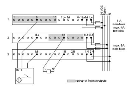
4-Wire Sensor with a 3-Wire Actuator
