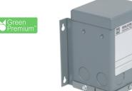
Transformer, buck boost, encapsulated, 0.05kVA, 1 phase, 120x240V primary, 16/32V secondary, NEMA 3R, 55C rise
