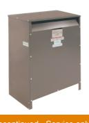
Transformer, dry type, 45kVA, 3 phase, 480V delta primary, 240V delta secondary, 18D, 150C rise, Cu
